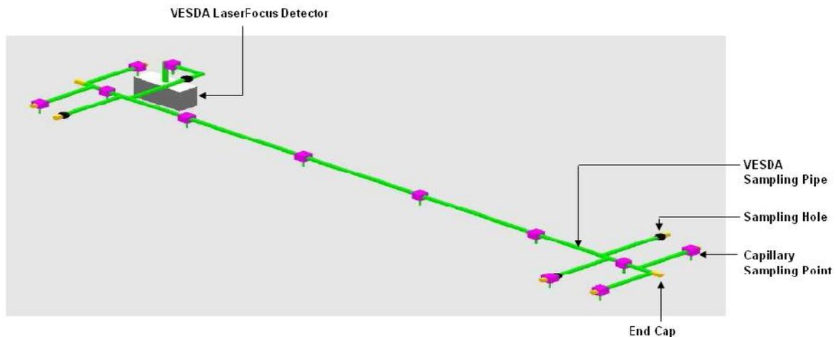
The typical arrangement of a concealed sampling point is shown in the diagram below.
