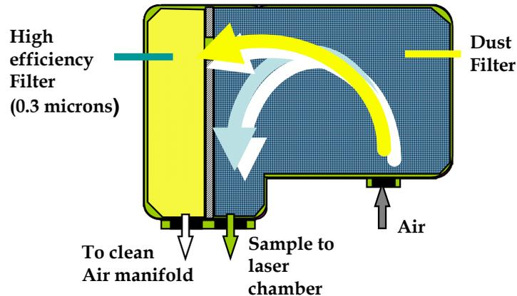
First stage of the filter removes dust and dirt from the air sample before the sample enters the laser detection chamber for smoke detection. The second (ultra fine) stage provides an additional clean air supply to keep the detector's optical surfaces free from contamination, ensuring stable calibration and longer detector life. The detector constantly monitors the filter efficiency and a fault is raised automatically on the detector when the filter needs to be replaced.
