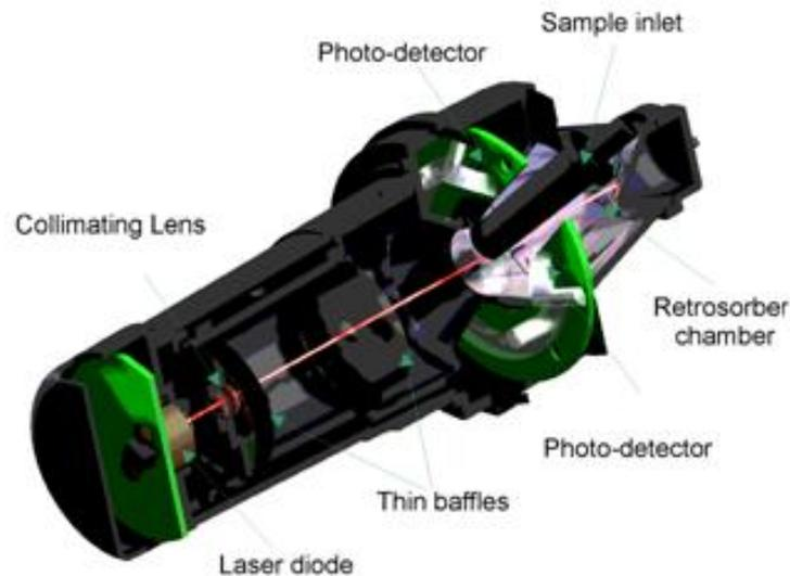
When smoke is present, the laser light gets scattered within the detection chamber that is detected by a very sensitive receiver system using sophisticated electronics. This signal is processed to represent the absolute level of smoke present. When the smoke density reaches the set threshold an alarm is raised.
