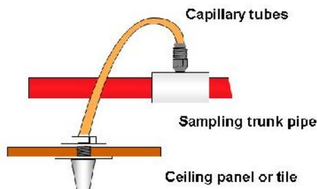
These sampling points are installed at locations with public (passengers) access - passage and seating area. Inside equipment cabinet, normal sampling holes are considered.
