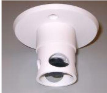
The HASP head operates on thermal detectors principle in its normal operating mode. As fire starts and develops, heat (ambient temperature) increases to such point that the sampling hole is opened and it becomes a normal air sampling hole, hence the detection of the fire and alarm from Xtralis VESDA detectors. As per the Certificate of Appraisal, issued by National Building Technology Centre of Australian Government, the heat activation temperature is 68 °C.
