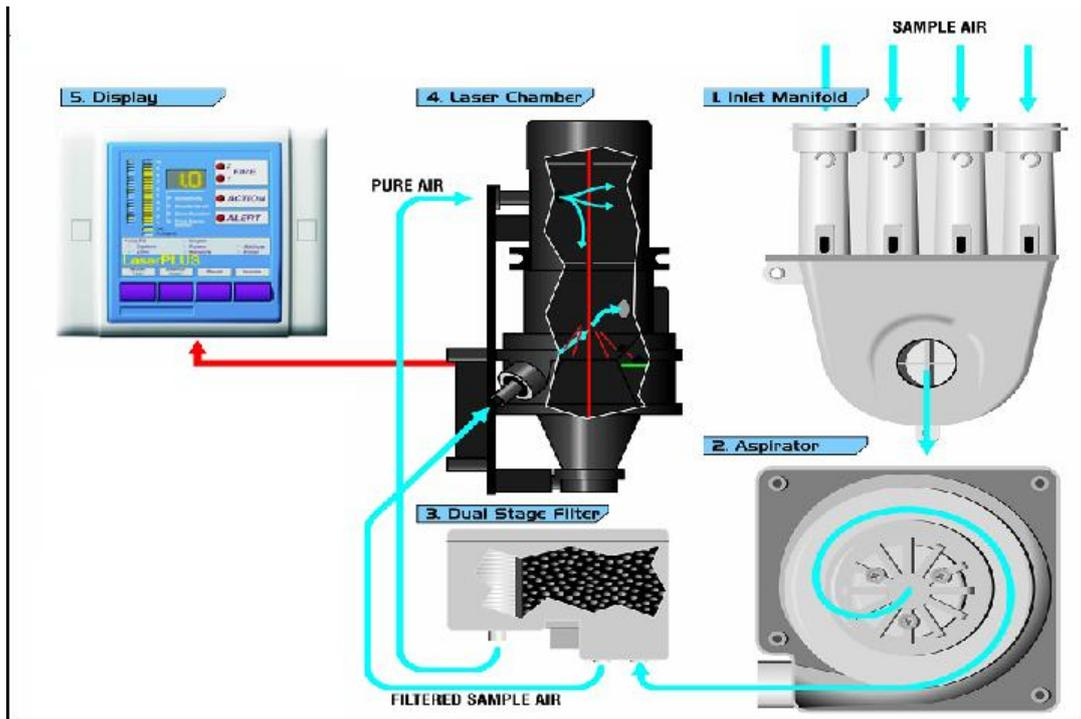
1. Air is sampled by the Xtralis VESDA detector through a pipe network specially designed to the requirements of the individual train coaches.
